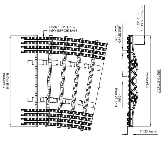
SilentFLOW DPAR: ALL COMPONENTS ARE CORROSION RESISTANT,
